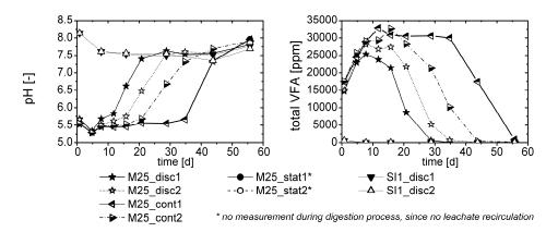
Figure 2 pH values and VFA concentrations in experiment 1 with a high proportion of readily degradable organic material (25% ensiled maize)
